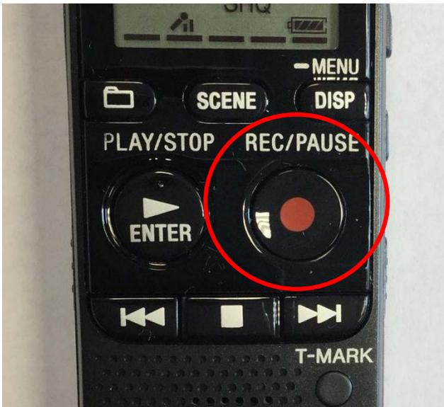
When you are finished recording, press the **STOP button** below the REC button. You will hear another small "beep," and the red light at the top will go off. Press the **REC button** to pause your recording. Press the **PLAY button** to playback what you've recorded so far.
