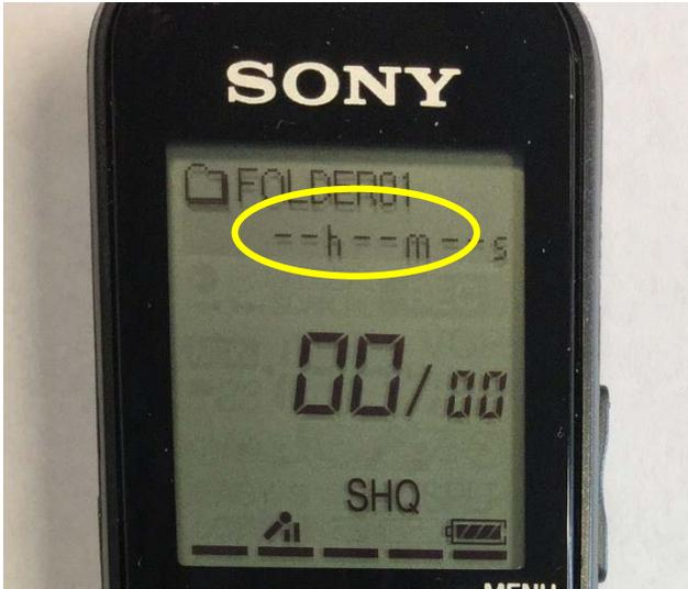
You generally want to begin recording into **Folder 01**, so simply press the **red REC button** below the screen to begin recording. You will hear a small "beep," and the red light at the top of the recorder should light up.
